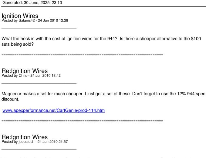
The cost is in te Beru fittings on the ends. These can be reused of you unscrew the ends and crimp on new screw ends. Then you re use the old beru fitting. I make my own plug wires like this.
